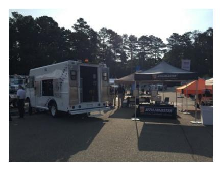
The 14' Utilimaster walk-in-van, designed, engineered, and manufactured specifically for Spartan Motors' customer Hawaiian Electric Company, is built on a Ford F-59 commercial chassis with a Kubota gas generator, Team Fenex air delivery system, and upfitted with EZ Stak interior cabinetry. This particular specialty service truck will be used to maintain and service the underground electrical infrastructure in Honolulu, Hawaii.
