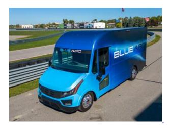
The Blue Arc portfolio includes Class 3 all electric delivery vehicles offering 600, 700 or 800 cubic feet of cargo capacity and up to 5,000 lbs of payload. The Class 4 offers 700 and 800 cubic feet, and Class 5 provides 900, 1110 and 1,200 cubic feet options and payload of up to 7,500 lbs.
